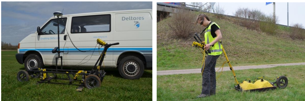
Figure 3.3 Unshielded 100 MHz antennae mounted on a cart (left) and 250 MHz shielded antennae in tow set-up (right).
