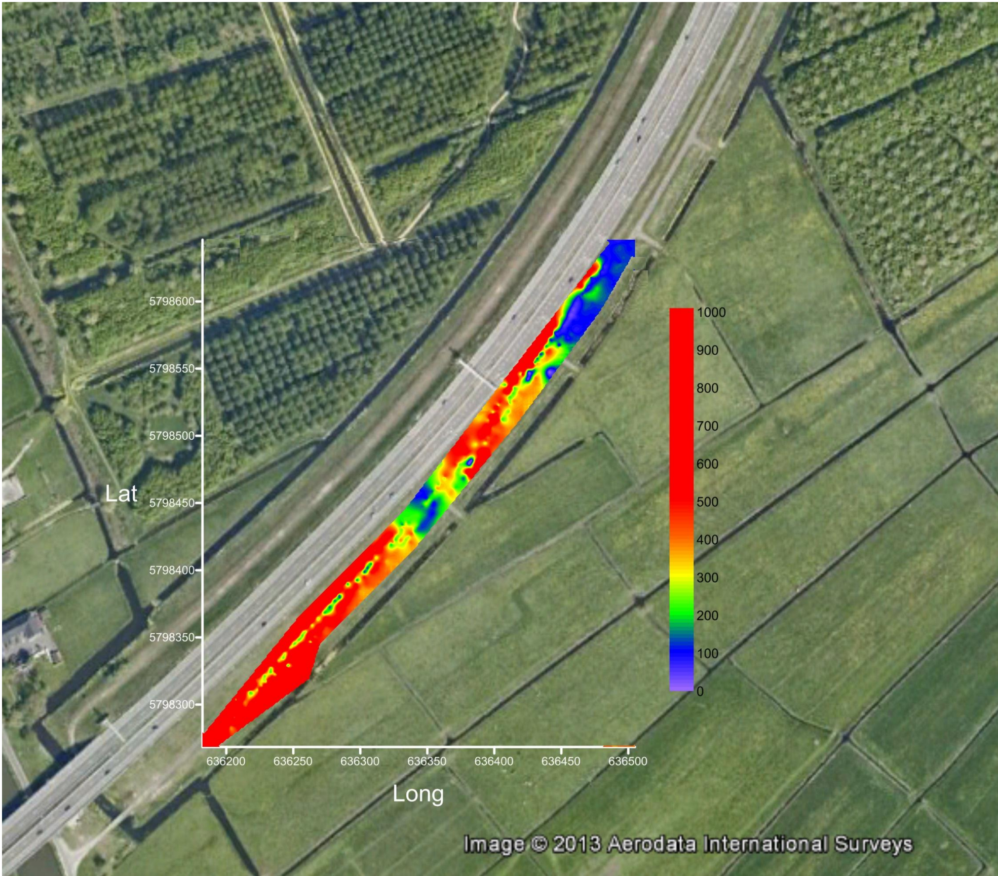
Figure B.10 Apparent resistivity values for Ohmmapper with transmitter-receiver distance of 5 m (sensitive to approximately 2 m depth).
