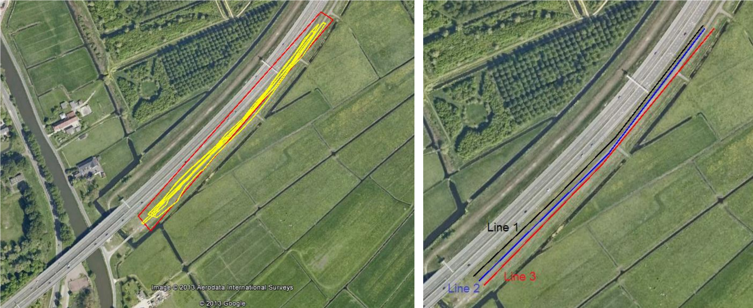
Figure B.9 Left: Location of Capacitive Resistivity Tomography survey lines using Ohmmapper (yellow lines). Right: location of inverted lines from Ohmmapper data.
